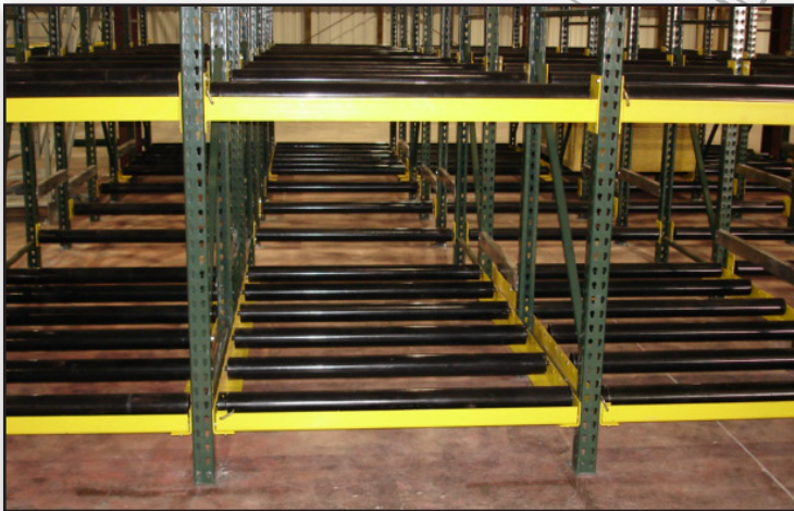
Rollers on 24" Centers to prevent Deflection
