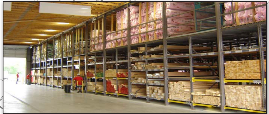
Interior Drive-Thru Auto-Stak Racking with Mezzanine above
