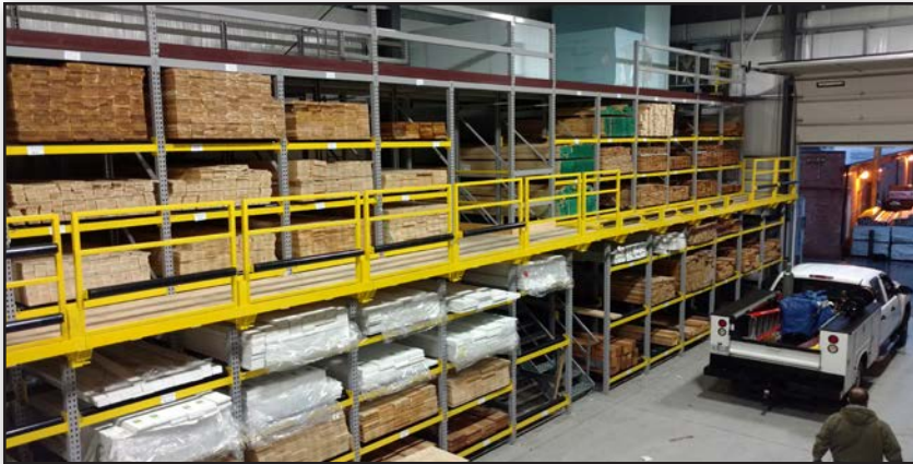
Auto-Stak with two Mezzanine Levels
