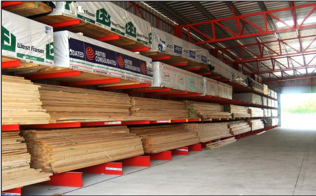
Single Face Cantilever within Drive-Thru Building
