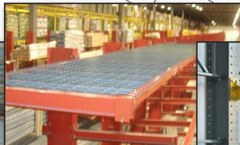
Beam Saddles & Decking
